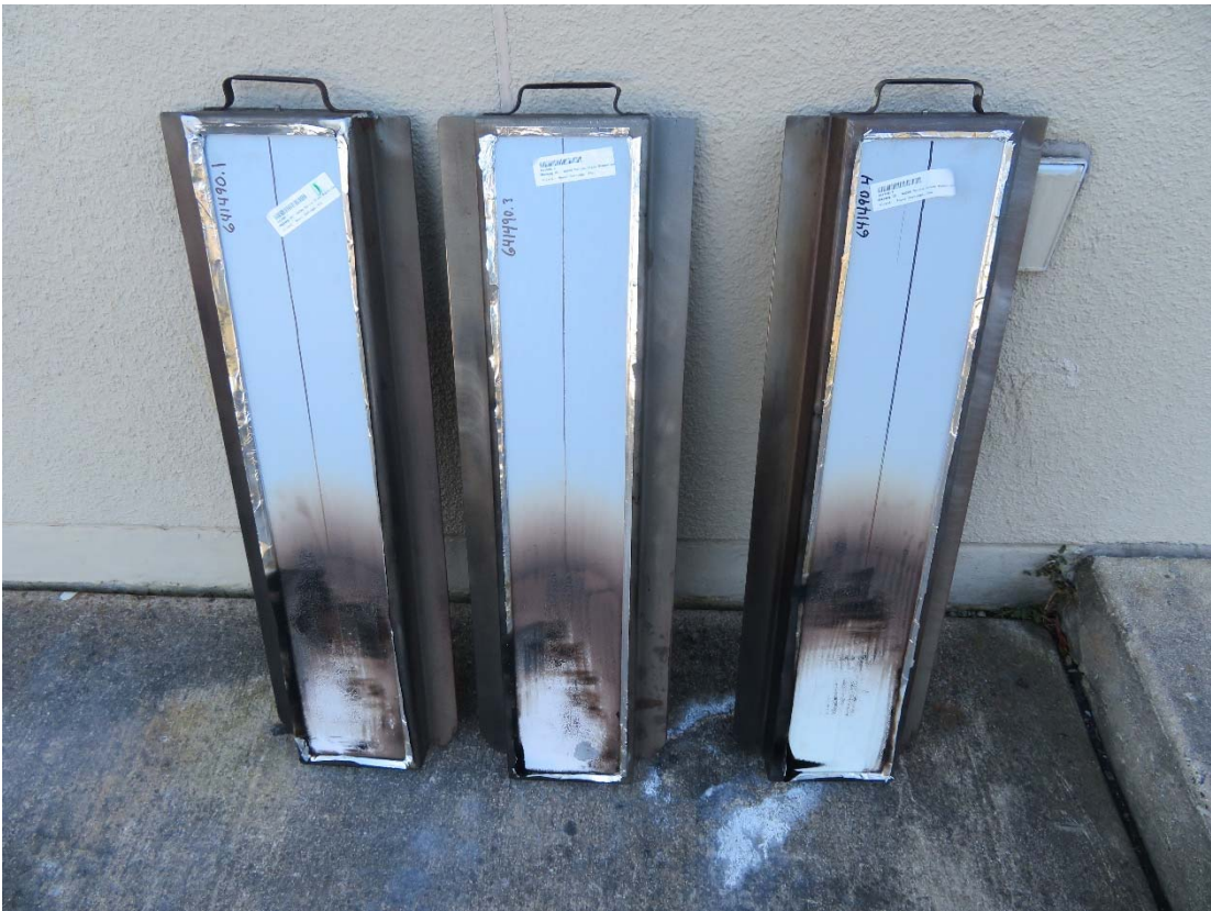
Figure B-3. Tests 1-3 (left to right) after fire exposure.
